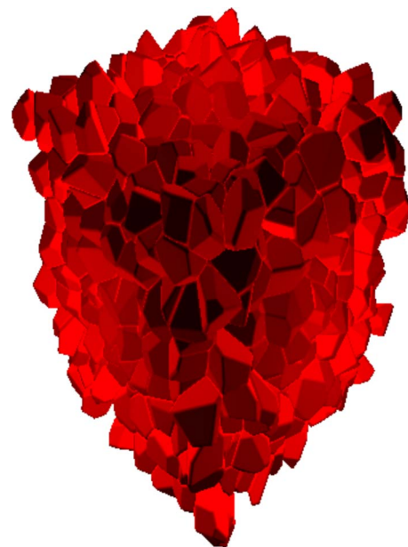
FIG. 8. (Color online) A three-dimensional array of Voronoi spheropolyhedra.
